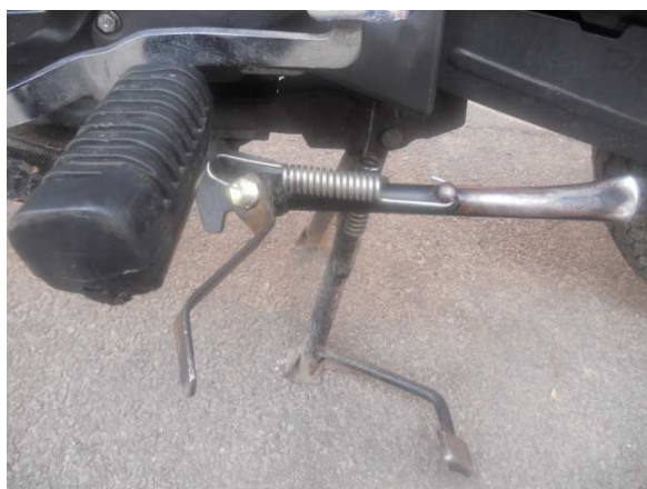
Figure 4: Released position of the side stand with assembled side stand lock link
