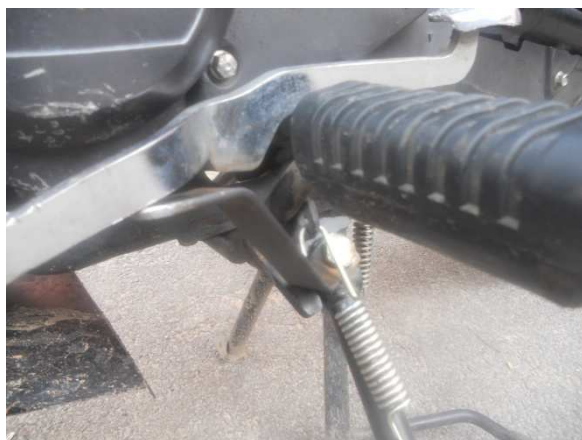
Figure 3: Closer view of unreleased position of the side stand with assembled side stand lock link
